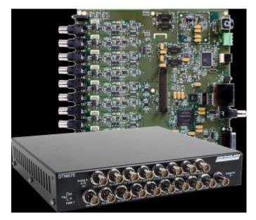
The DT9857E offers many capabilities for vibration measurement such as 16 IEPE 24-bit Delta-Sigma sensor inputs, two 32-bit D/A stimulus outputs, a 32-bit tachometer, pre- and post-triggering.
